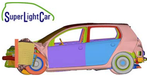
Fig. 5 ODB crash of the SLC vehicle
