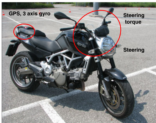
Fig. 6 The UNIPD instrumented motorcycle
