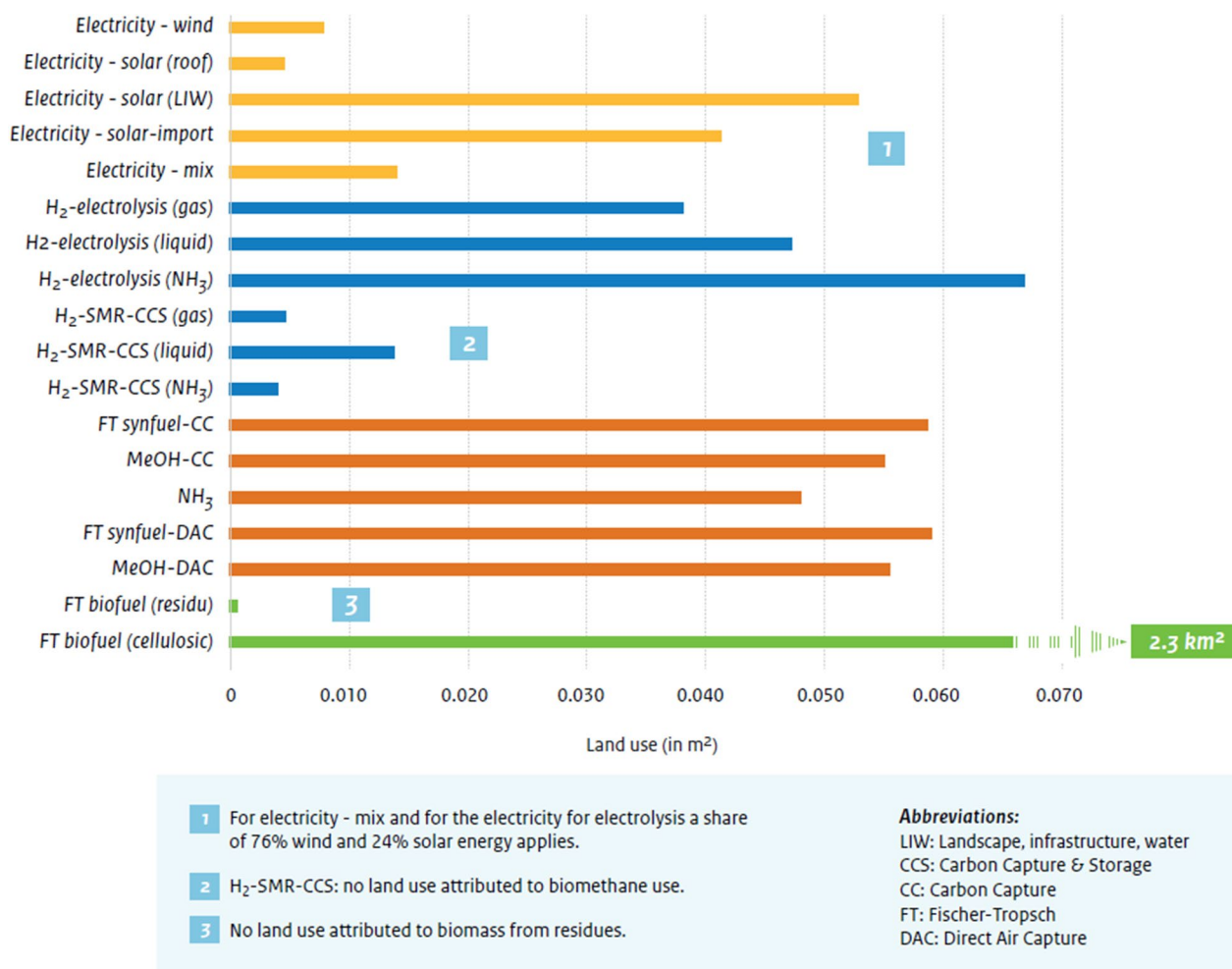
Fig. 2 Net land use of energy supply for 1 inland vessel (Large Rhine class vessel, 110 m).
